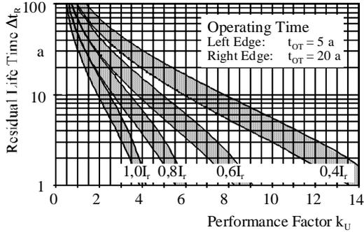
Fig. 11. Residual Life Time of Al/Al-Joints Depending on the Performance Factor
