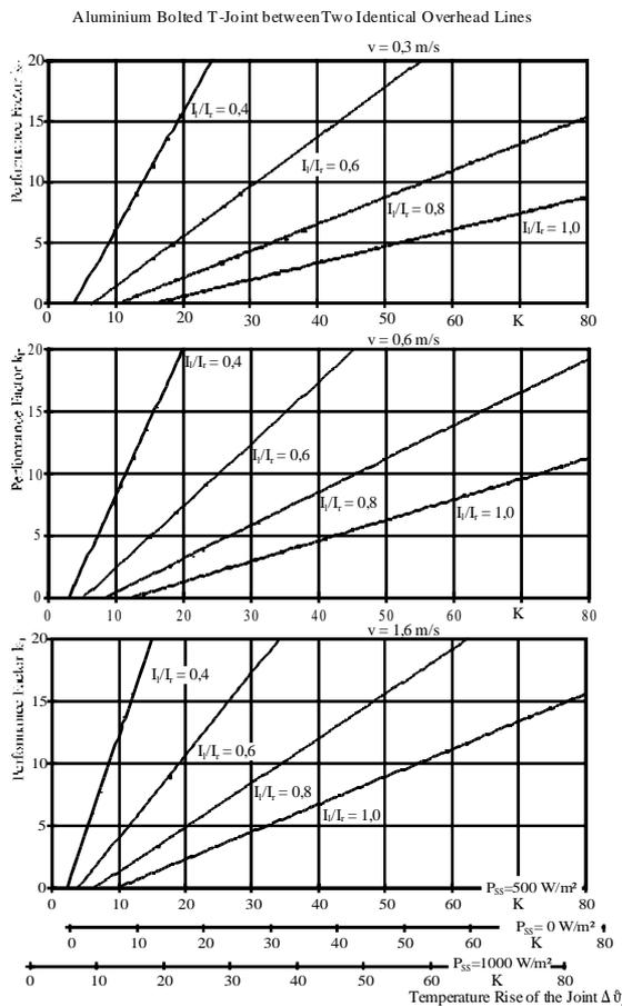
Fig. 10. Determination of the Performance Factor out of the Temperature Rise of the Joint
