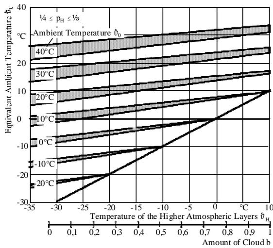
Fig. 4. Equivalent Ambient Temperature Depending on the Higher Atmospheric Layers
