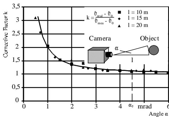
Fig. 2. Thermal Resolution Angle of an IR Camera
