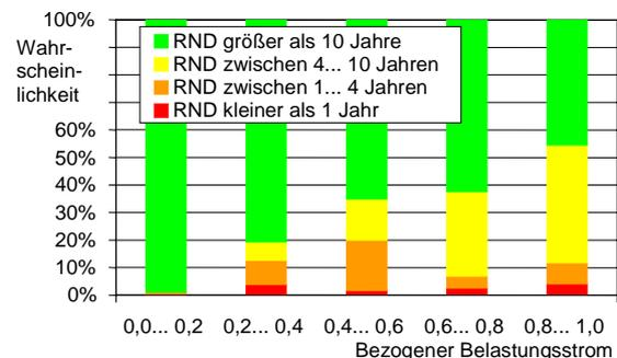
Fig. 17. Probability of the Determined Residual Life Time Depending on the Related Load Current
