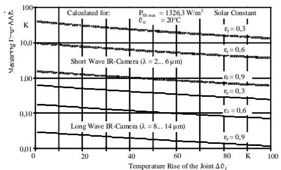
Fig. 3. Measuring Error Depending on Solar Radiation
