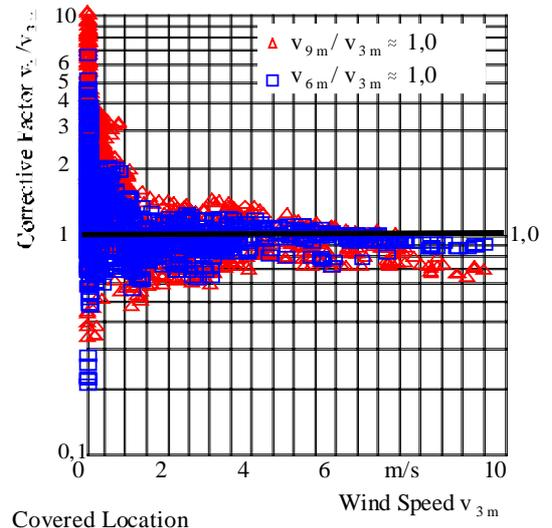
Fig. 8. Wind Speed Depending on the Height
